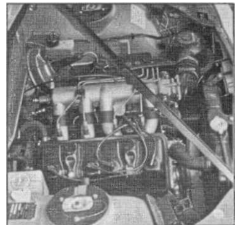
Above: The forward two induction pipes are curved to clear the distributor; a very large oil-bath air cleaner is used. Below: The side lamps and indicators are shaped to complete the composition at the front.
