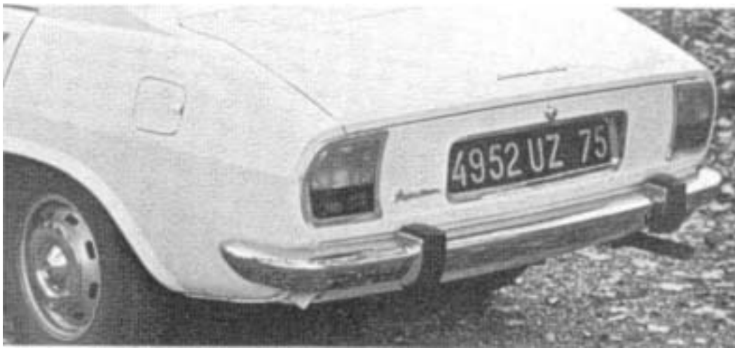
Rubber-faced over-riders are another sensible and practical feature. Wheel trims are held by a centre bolt and not dipped on as on other cars
